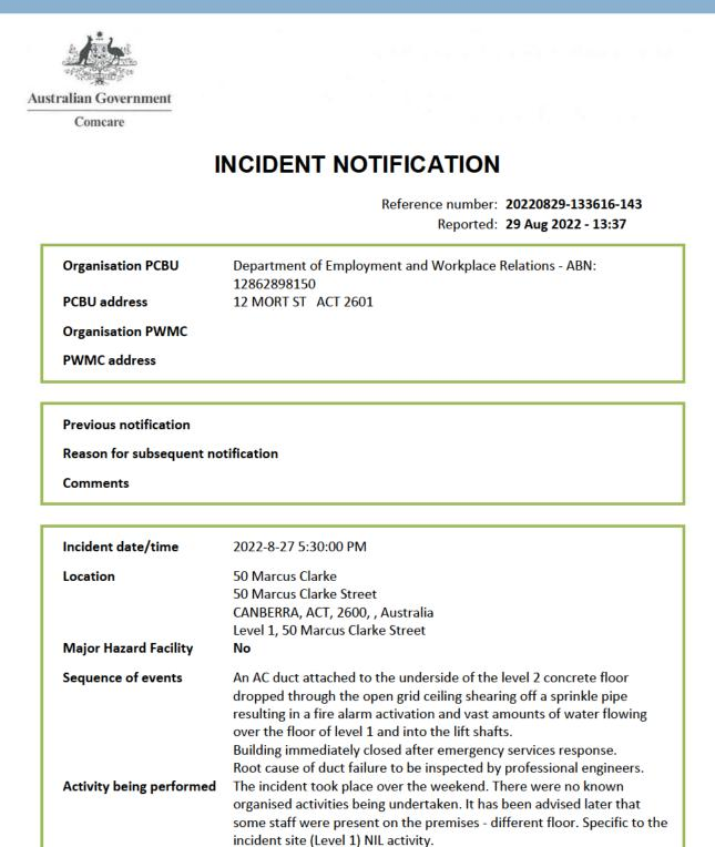
Items involvedAC duct, aluminium decorative ceiling grid, fire sprinkler systemType of incidentDangerous Incident - The fall or release from a height of any plant,
